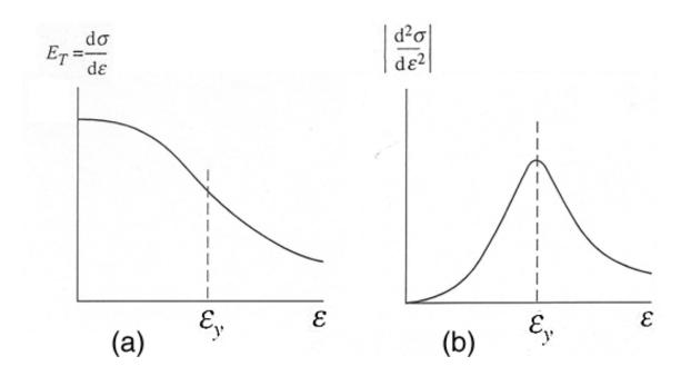
Fig. 2 Derivatives of stress strain curve
