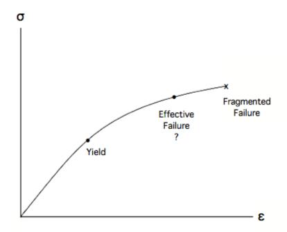
Fig. 6 Failure stress possibilities
