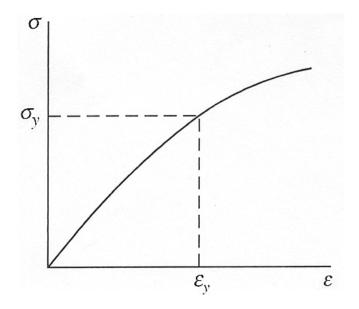
Fig. 1 Stress strain curve
