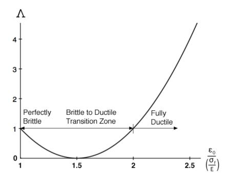
Fig. 9 Energy dominance versus failure strain
